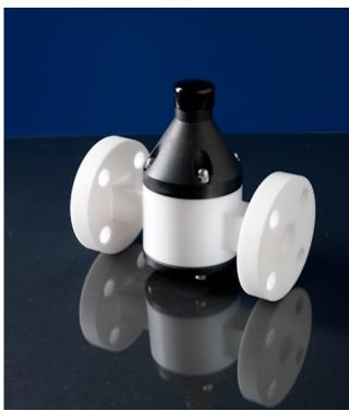
**Griffco G-Series** diaphragm back pressure valves are designed to enhance the performance of chemical feed systems by applying a continuous back pressure to the chemical feed pump, while also acting as an anti-syphon valve. Robust construction ensures reliability in the rigorous service of sulphuric acid for both municipal and industrial applications. Wetted materials are: **PTFE.** Available sizes: 1/2" - 1".
