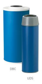
Pentair UDS & DBC Series Cartridges are enhanced with KDF media to inhibit scale buildup that can damage equipment. These cartridges are constructed of high performance granular activated coconut shell carbon and a 5-micron spun bonded polypropylene post sediment element for increased dirt holding capacity. They are effective for chlorine taste and odor reduction in high capacity situations and where lime and scale buildup problems occur.
